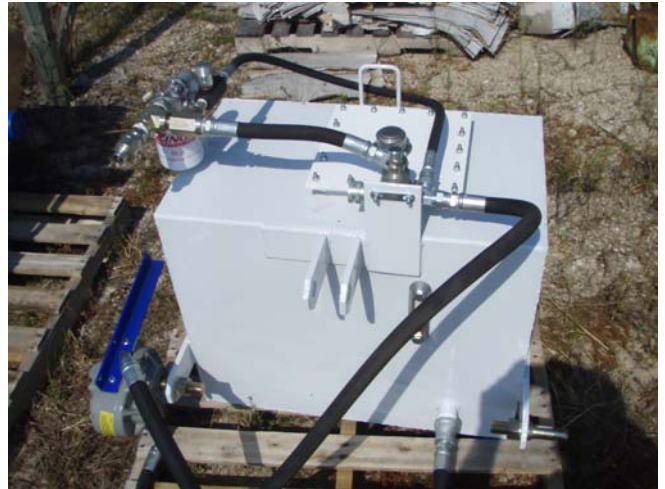
Hydraulic Tank to run collector
