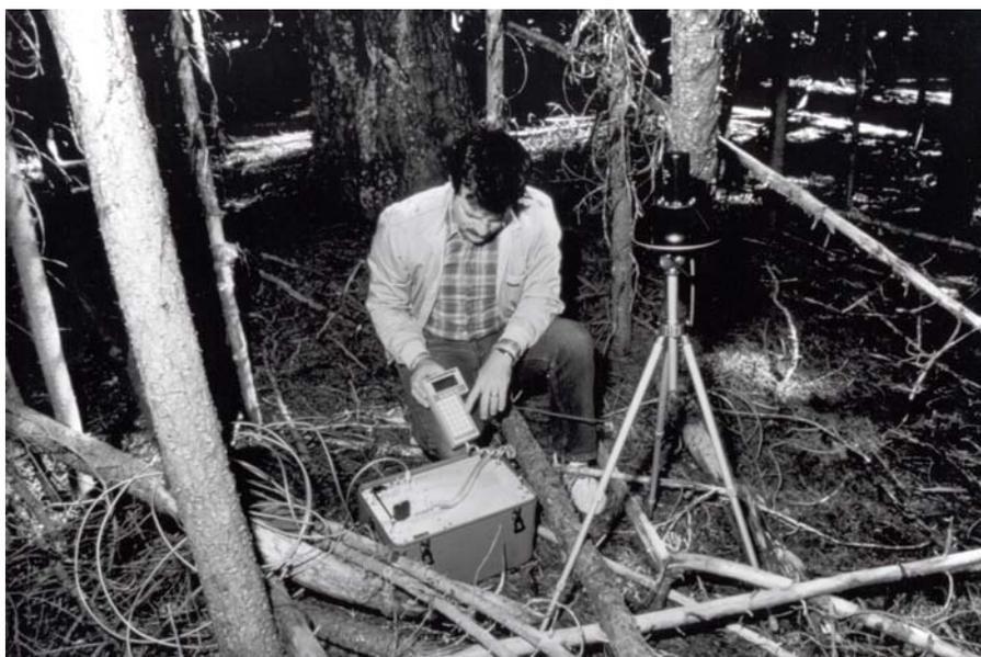
Figure 3—The first GPS receivers were large, heavy, and power hungry.
