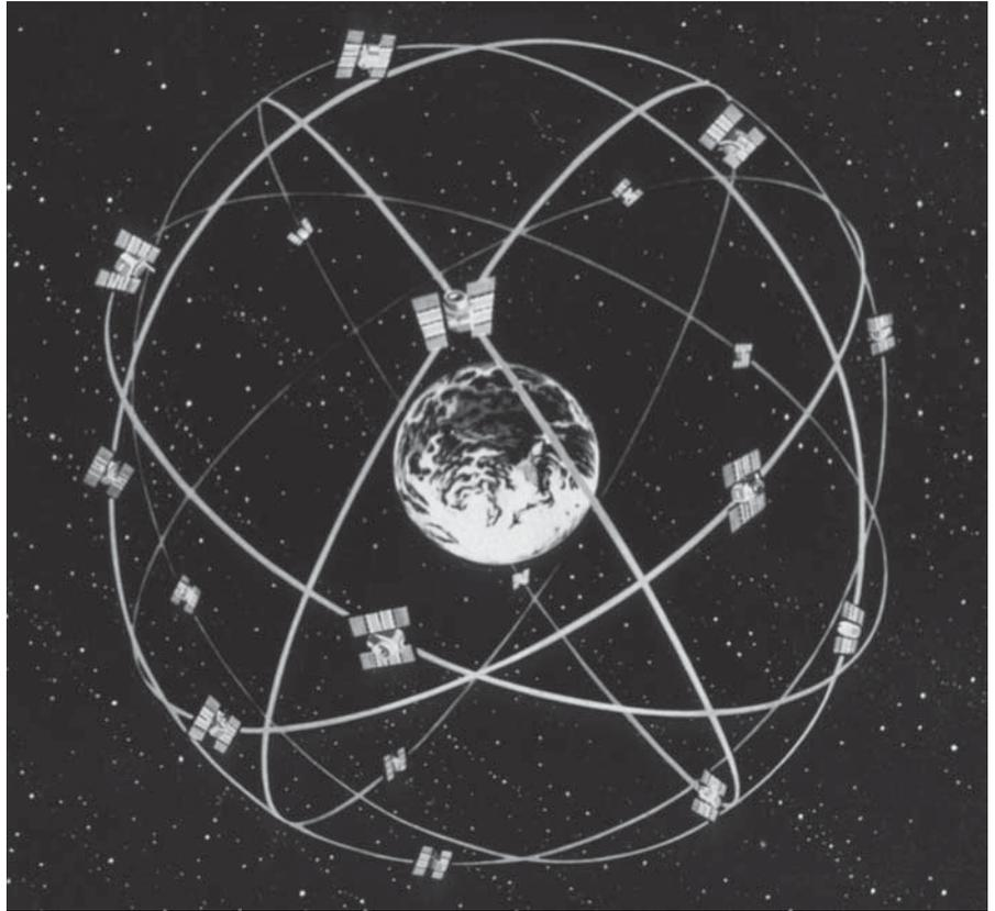
Figure 1—The operational GPS satellite constellation consists of 24 NAVSTAR satellites arranged in six 55° planes around the Earth so that a minimum of four satellites would always be in view above the horizon.
