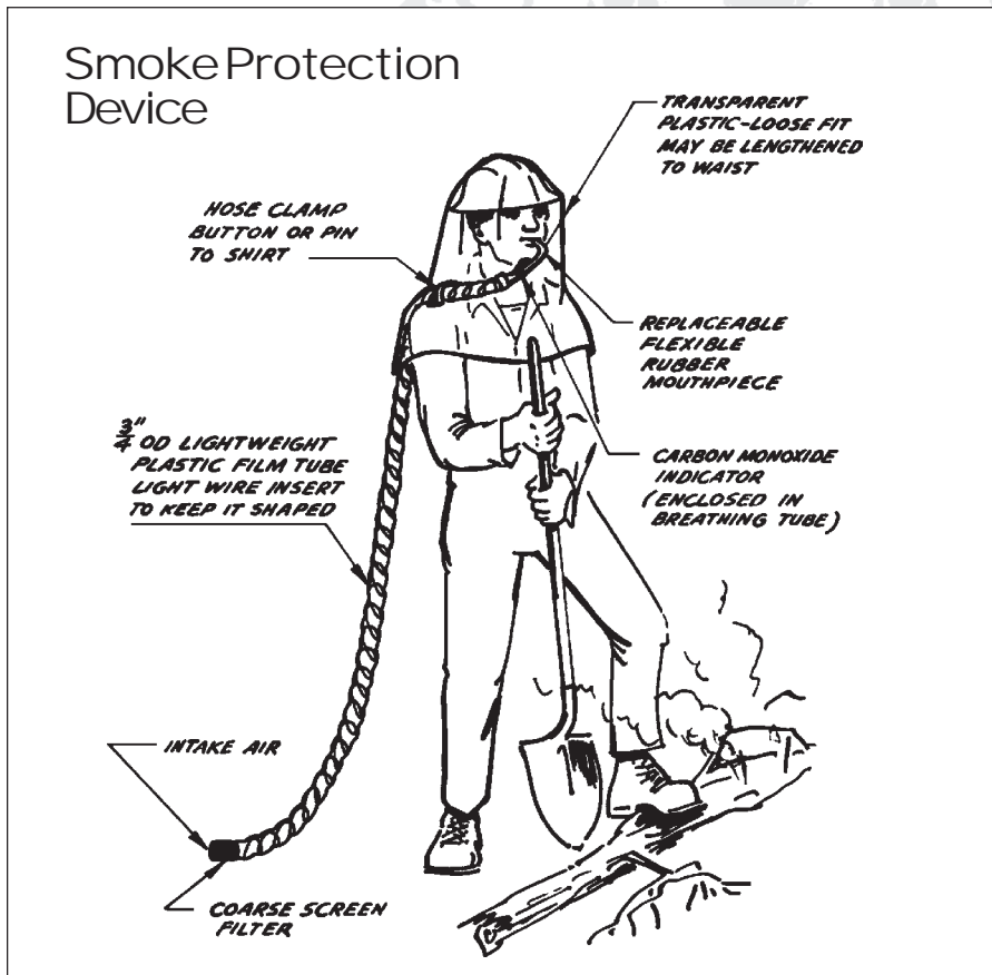
Employee suggestion (circa 1960) for a respiratory protection device.
