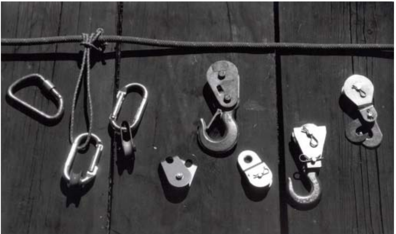
Figure 4.—Useful hardware for hoists.
