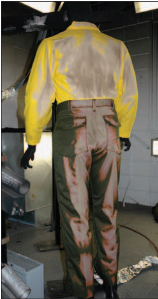
Figure 8—Large portions of the aramid shirt and pants changed color—a sign of exposure to high levels of heat—after the radiant heat test.
