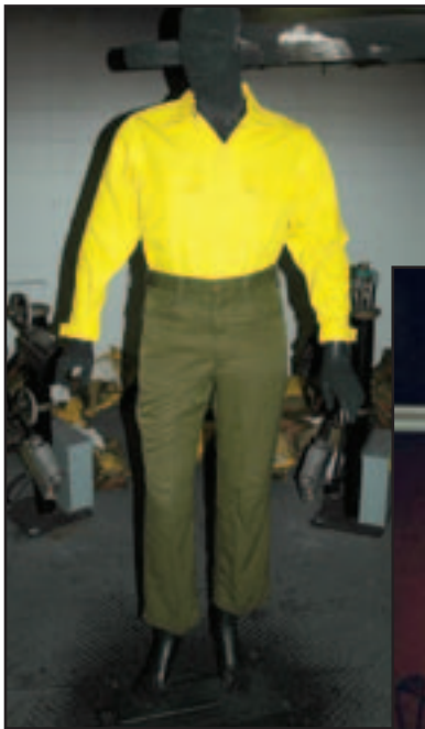
Figure 2—The mannequin was outfitted with a flame-resistant aramid shirt and pants before testing.
