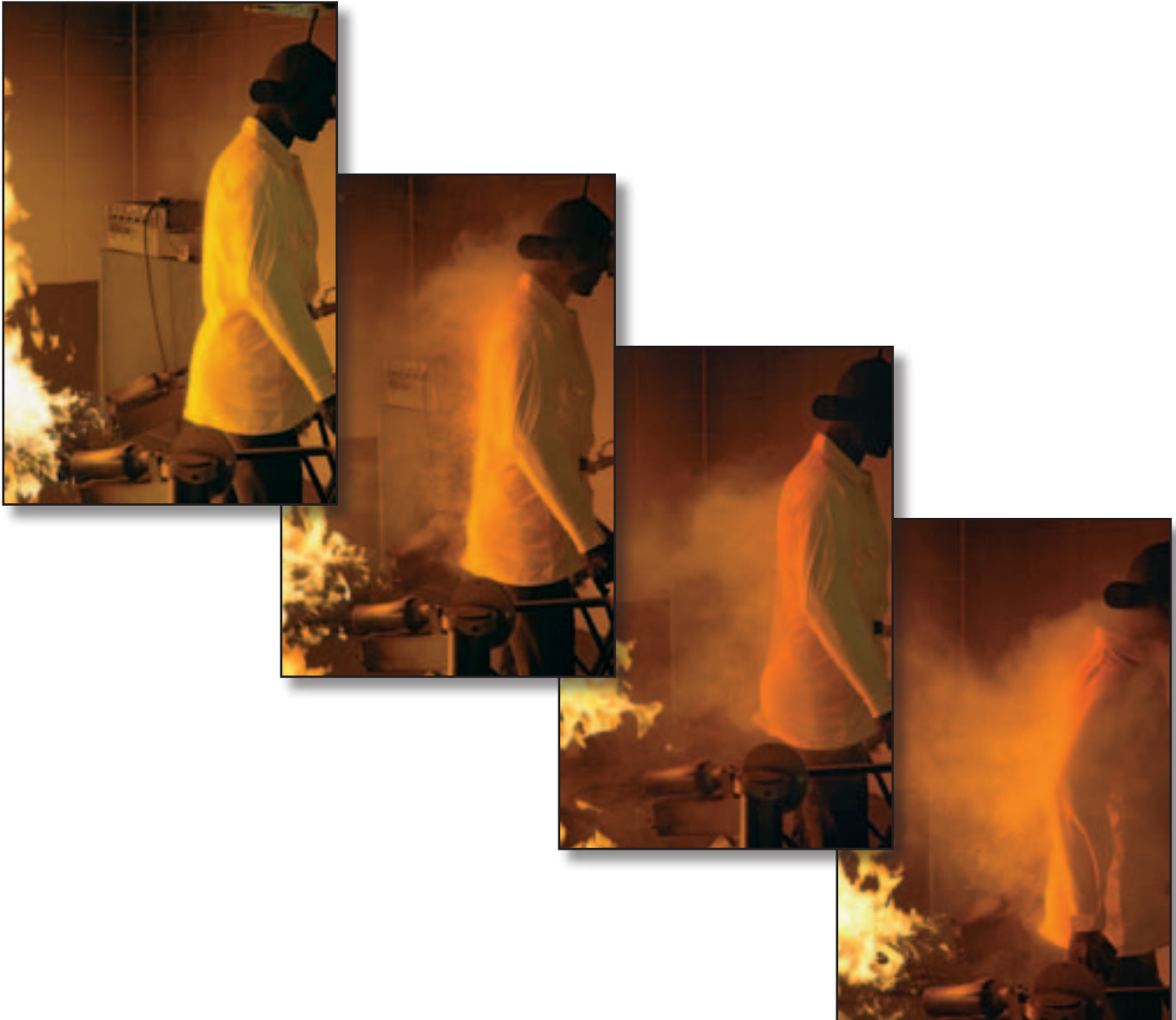
Figure 7a, 7b, 7c, and 7d—The aramid shirt showed the effects of heat throughout the 10-second radiant heat test.
