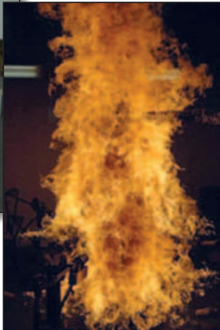
Figure 3—The mannequin is fully engulfed in flames during the full-scale flame engulfment test.
