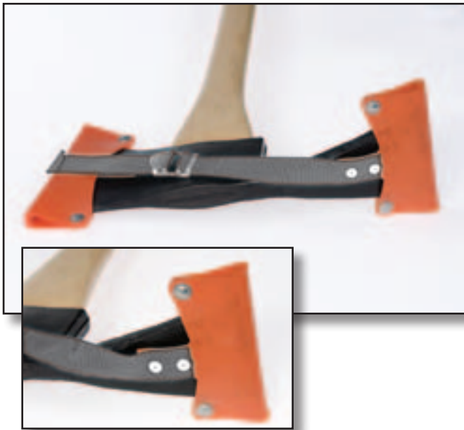
Figure 4—Rivet (inset) the 1-inch-wide webbing to the plastic strap.
