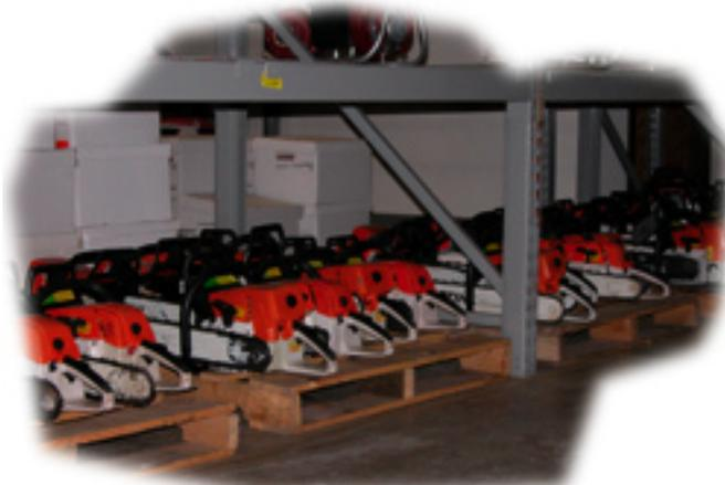
Figure 2—After cleaning a saw or other tool, it's a good idea to dry it and wipe it with light oil or a water-displacement product, especially if the tool is going to be stored.
