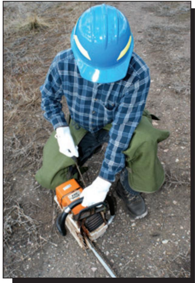
Figure 3-17—Start the saw on firm ground.
