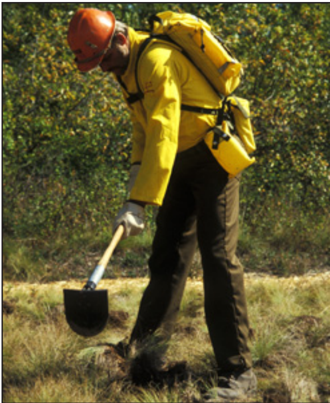
Firefighters using a Combi tool rather than a pulaski produce more fireline for each liter of oxygen consumed.
