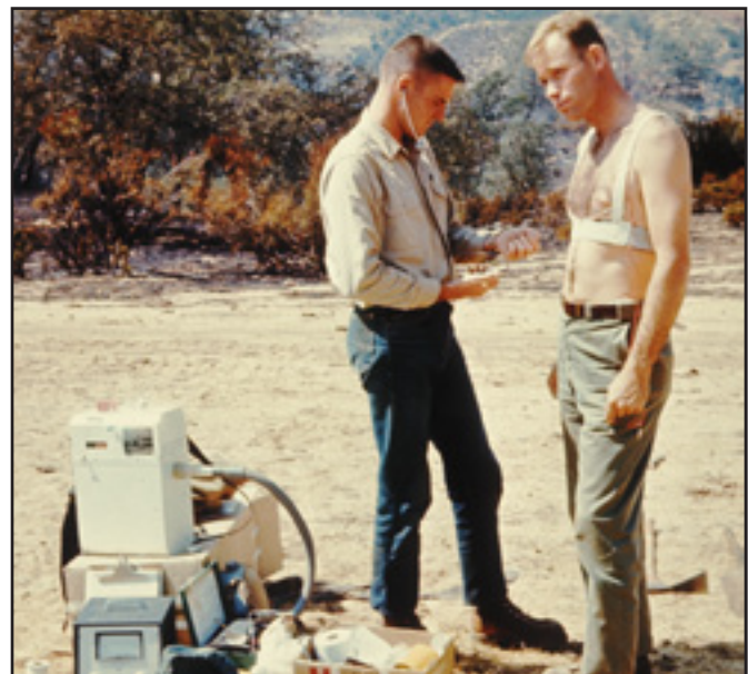
In this 1965 photograph, MTDC employee Cliff Blake is a subject during a study of energy, cardiovascular, and thermal demands of wildland firefighting.
