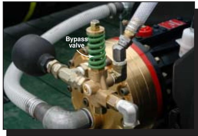
Figure 9—A bypass valve directs water back to the holding tank when water is not needed for the wands or underbody washers. This valve will prevent damage to the pump, but its internal parts can wear and require replacing. Hydraulic fittings make the valve easier to replace.
