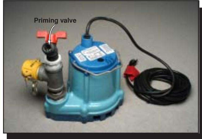
Figure 17—The mat sump pump has a valve attached to the outflow. This valve is used to prime the pump. Opening the valve allows water to flow through the pump without any head pressure. Once the flow is established, the valve is closed and water is pumped to the settling tanks.
