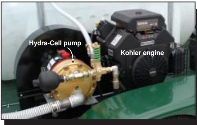
Figure 8—A high-pressure and high-volume diaphragm pump provides water to the wash wands and underbody washers. A 25-horsepower, two-cylinder engine powers the pump.
