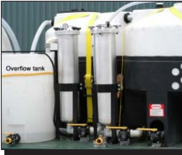
Figure 11—Overflow from the settling tanks flows to the overflow tank (left). A sump pump inside the overflow tank pumps water through two filter housings to the holding tank. The filter housings use polypropylene or polyester felt and nylon monofilament filters to remove particulate of different sizes, depending on the user's requirements. The size of particulate filtered can range from 800 microns to as fine as 3 microns.
