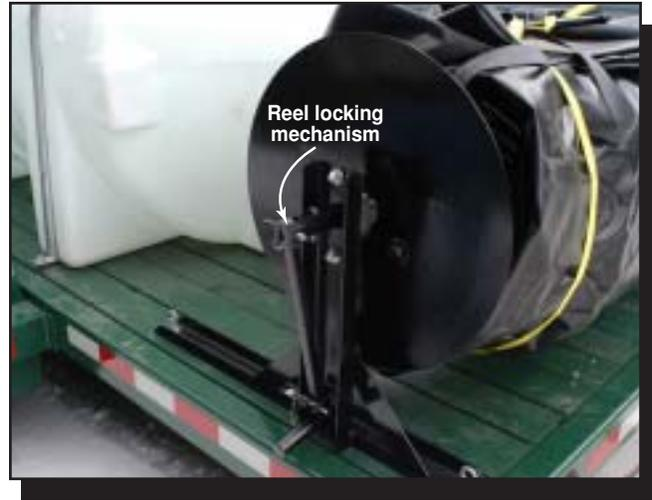
Figure 14—The mat reel's locking mechanism prevents the mat from unrolling accidentally.
