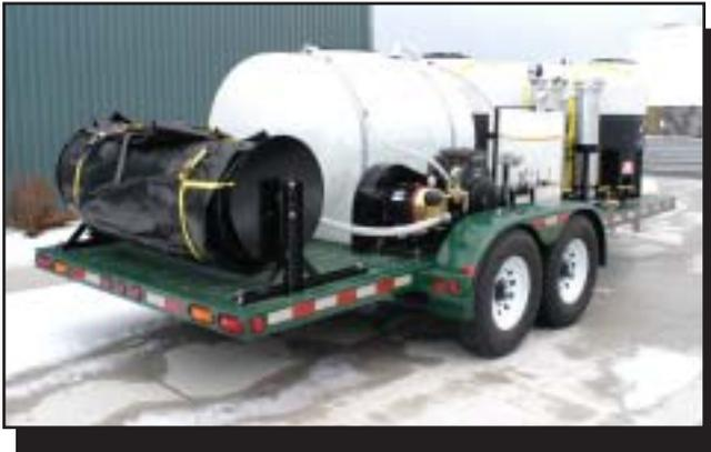
Figure 13—The mat reel is used to roll up the mat for transportation and storage.
