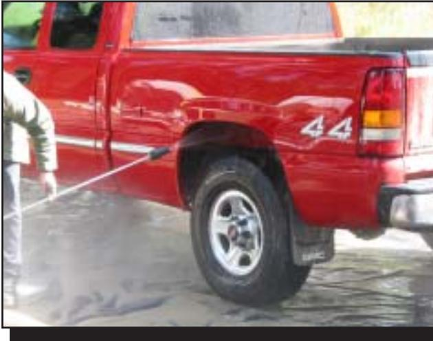
Figure 4—The hand-operated, high-pressure wands are used to clean mud, dirt, spores, and weed seeds from a vehicle’s wheel wells, tires, sides, and bumpers.
