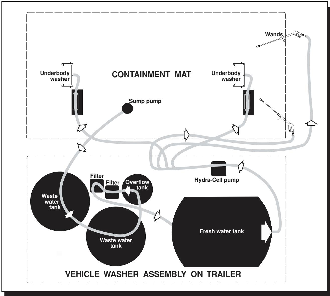
Figure 3—The flow of water through the vehicle washer system.
