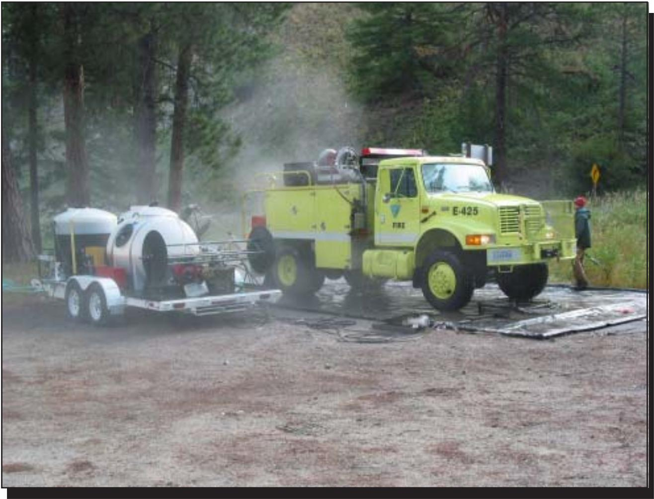
Figure 2—The MTDC portable vehicle washer being used in the field.
