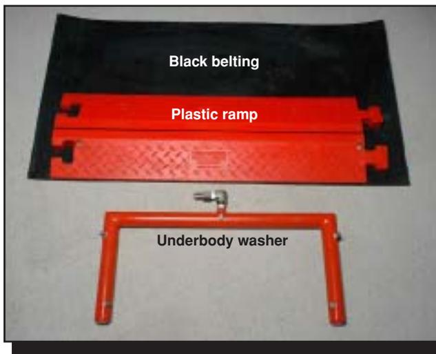
Figure 5—The underbody washer uses high pressure and a large volume of water to wash mud, dirt, and debris from underneath the vehicle. Nozzles are mounted so that they provide complete coverage under the vehicle. The ramp protects the hose that supplies water to the underbody washer. One underbody washer cleans vehicles as they drive onto the mat and another cleans them as they drive off.
