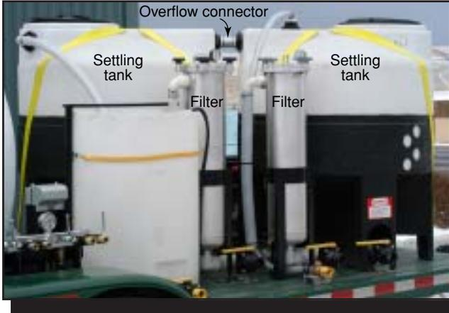
Figure 10—Two cone-bottomed tanks (background) are used as settling tanks to remove the larger particulate. Used wash water from the mat flows to these tanks before it is filtered.
