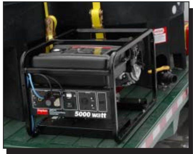
Figure 12—A 5,000-watt gasoline generator supplies power for the two sump pumps and can provide power for other electrical needs.
