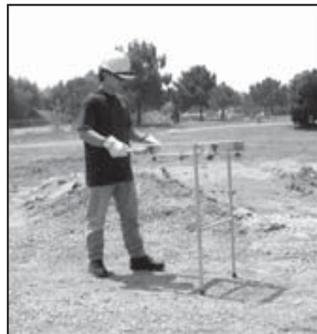
Alternative screens of different mesh sizes can be rolled up and carried with the kit. San Dimas will fabricate the screens.
