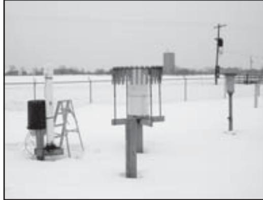
The Tech Tip, *Windshields for Precipitation Gauges and Improved Measurement Techniques for Snowfall* (0225-2325-MTDC), describes various windshields and their precipitation catch efficiency at different wind speeds. Some researchers have begun to abandon the bucket-type precipitation gauges that are protected by windshields. A hotplate snow gauge that melts snow as it hits the plate does
