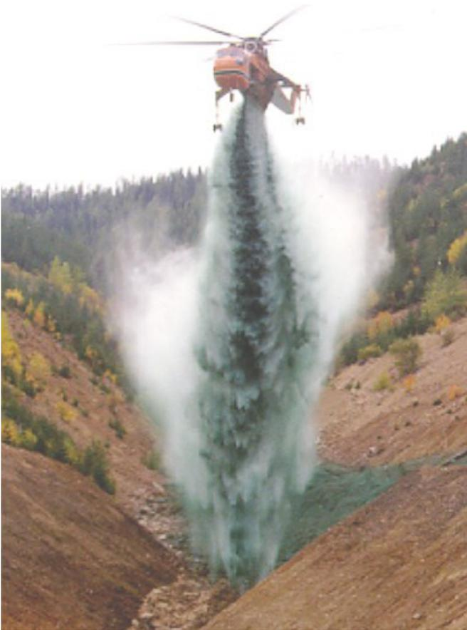
Figure 2—Aerial hydroseeding enables precise application on almost any terrain but the amount of material required necessitates expensive, specialized equipment.
