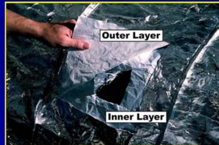
Slide 27: Photo: Outer and inner layers of the shell as well as seams of the shelter.
