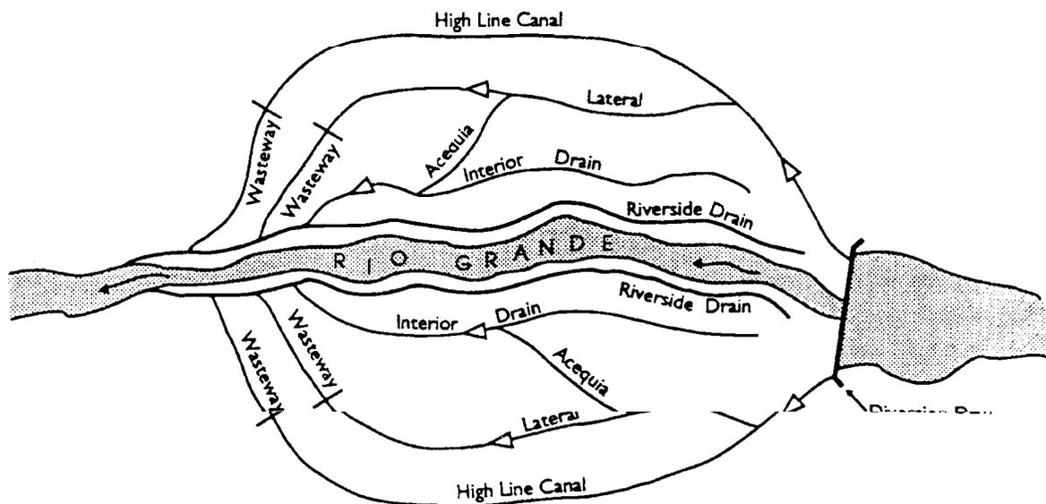
Figure 8. Schematic map of an irrigation network on the Middle Rio Grande (Bullard and Wells, 1992).
