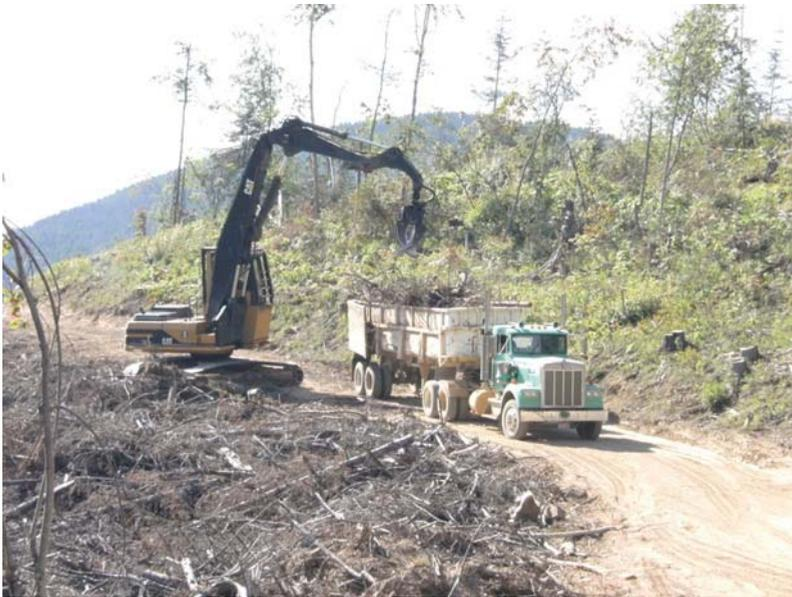
**Figure 14.4** An end dump semi-trailer used to haul slash to a concentration yard. (Photo: © Anderson, 2013).
