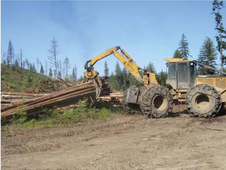
**Figure 14.5** Conventional grapple skidder releasing a turn of small diameter logs. (Photo: © Keefe, 2013).
