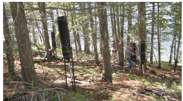
Fig. 2 Installation of ion exchange resin TF collectors near Boulder Lake (site—BLO). Snow tubes were attached to the collector funnels to allow for collection of snow in the winter season
