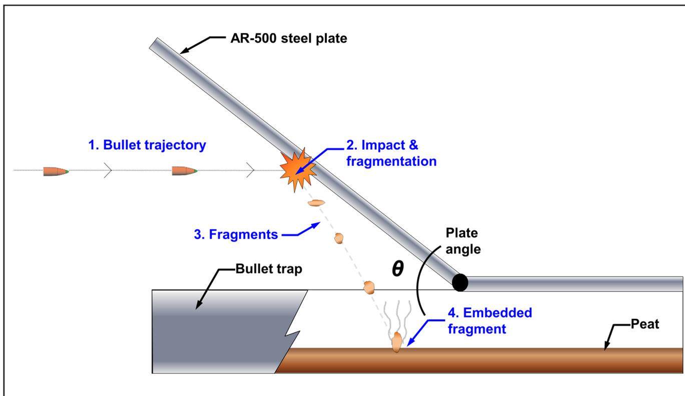
Figure 1—Experimental setup.
