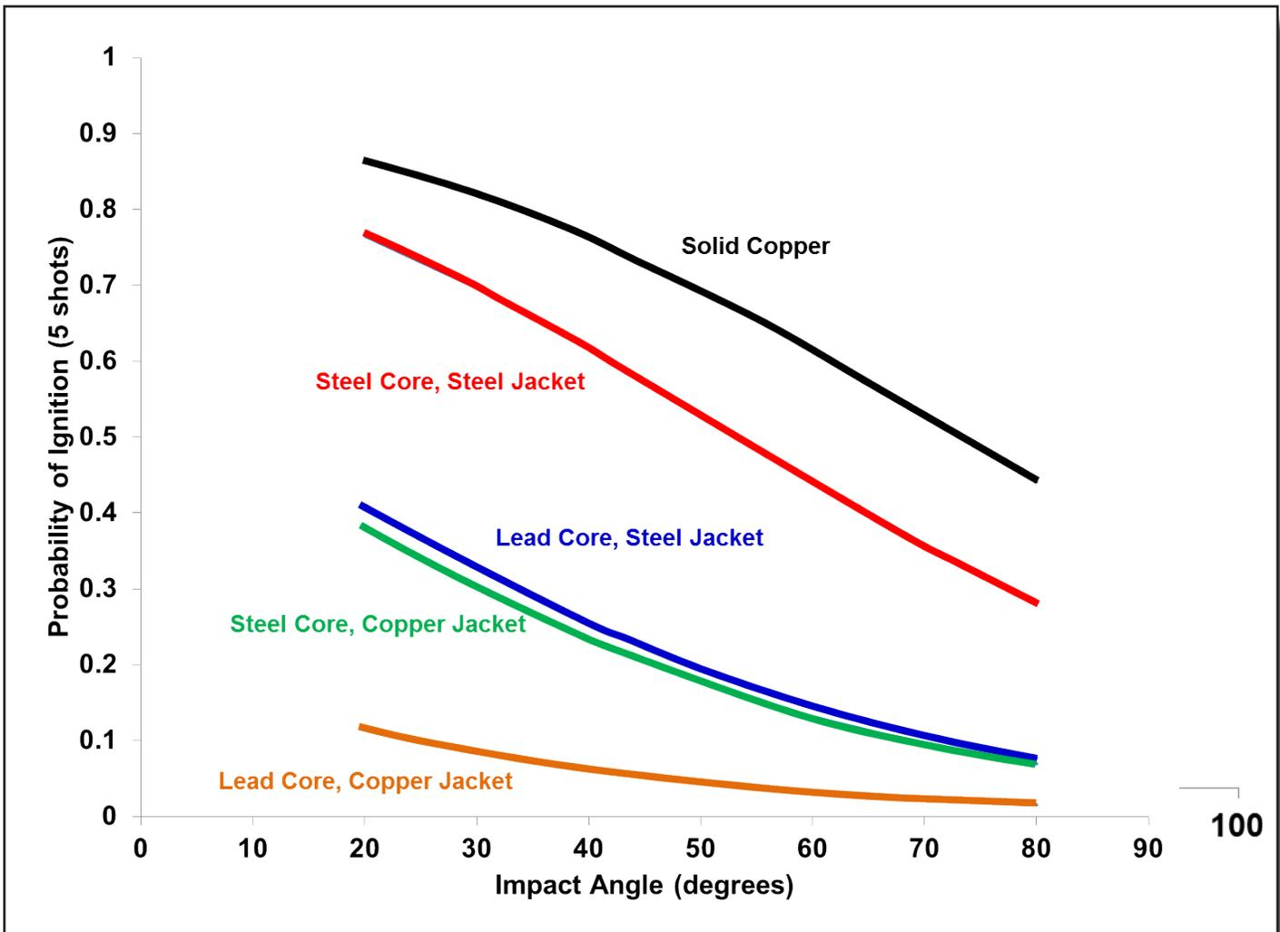
Figure 3—Probability of ignition for various bullets used in the experiment. Impact angle was varied by changing the angle of the steel plate. This probability of ignition applies only for the experiments described here.
