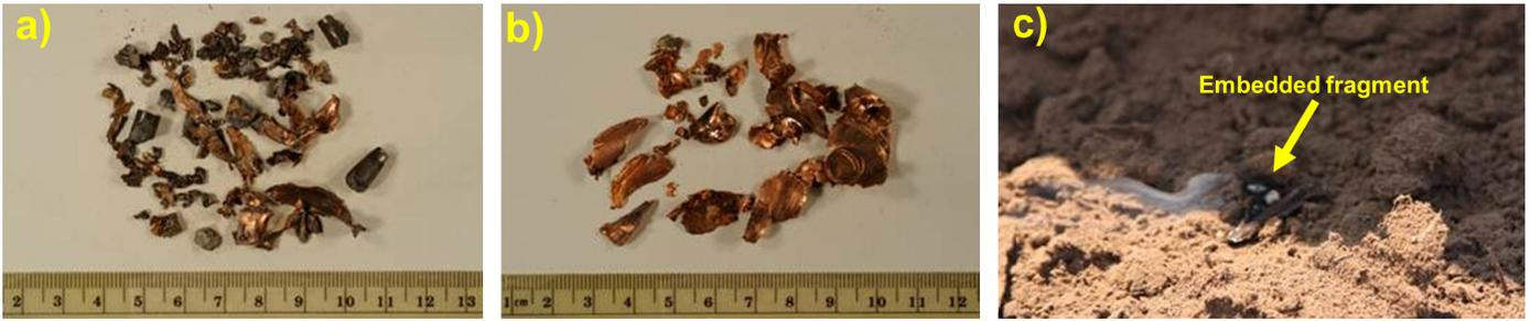
Figure 2— (a) Fragments from 7.62 by 54R steel core/steel jacketed bullet; (b) Fragments from 7.62 by 51 solid copper bullet; (c) Example of smoldering ignition from embedded bullet fragment.
