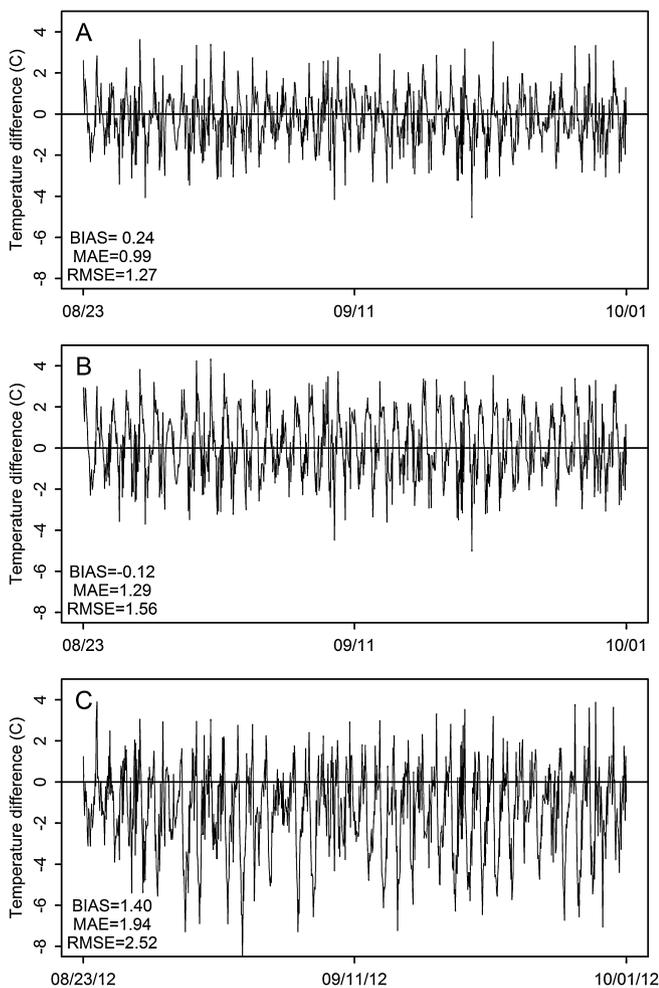
**Fig. 5.** Mean hourly temperatures differences between inexpensive radiation shield/sensor pairs and the Missoula NWS station. (A) NWS temperature minus radshield/Logtag; (B) NWS temperature minus Onset Gill-style/Logtag; (C) NWS temperature minus funnel/iButton observations.
