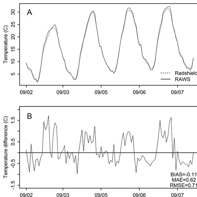
**Fig. 3.** Hourly temperatures measured at the Ninemile RAWS station and mean hourly temperatures recorded by three radshields and Logtag sensors. (A) Hourly temperature observations. (B) Differences in temperature between the RAWS and radshield (RAWS minus radshield).
