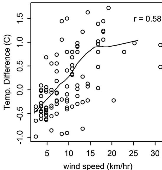
**Fig. 4.** A scatterplot showing the correlation between wind speed and radshield/Logtag and RAWS temperature observations (RAWS minus radshield).
