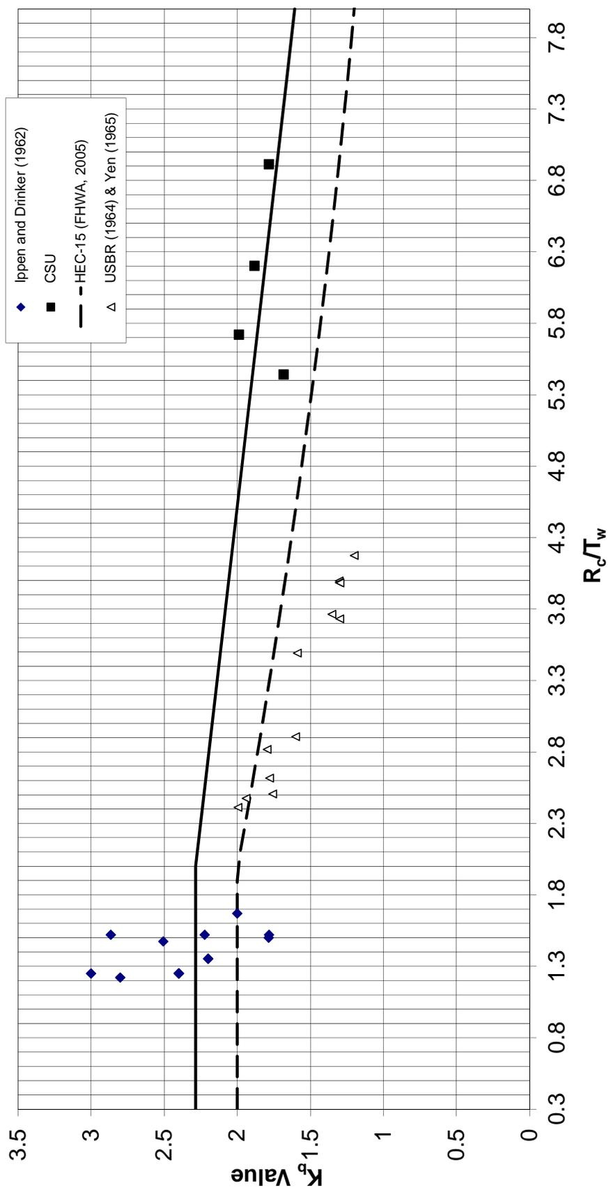
Figure 3.2: Best-fit Relation for Determining  $K_b$ , Using Only the Ippen and Drinker (1962) and CSU Data (Approach 1)
