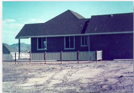
This landscape conserves water, but will make the house hot and cause erosion problems.
