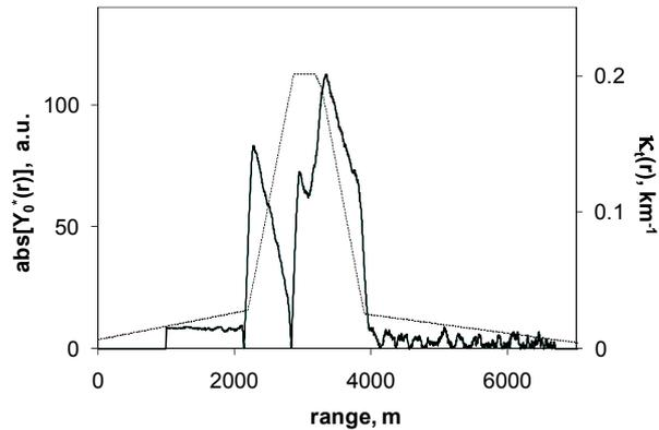
Fig. 1 – Model profile of the smoke-plume extinction coefficient,  $\kappa_i(r)$  (the dotted curve), and the corresponding normalized function  $|Y_0^*(r)|$  (the thick solid curve).
