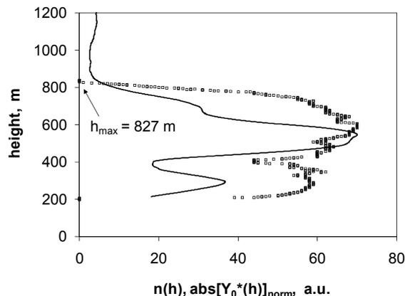
Fig. 3 – Heterogeneity Height Indicator for the case shown in Figure 2 (the empty rectangles) and the corresponding normalized profile of  $|Y_0^*(h)|$  (the thick solid curve).
