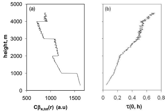
Fig. 6 – Model profiles  $C\beta_{\pi,tot}(h)$  and  $\tau(0, h)$  [the panels (a) and (b), respectively] used for simulations with different ratios  $C_{est}/C$ .
