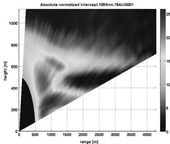
Fig. 2 – Heterogeneity Range-Height Indicator retrieved from the scanning lidar data at 1064 nm during the Tripod Complex Fire in the Washington state on August 19, 2006.
