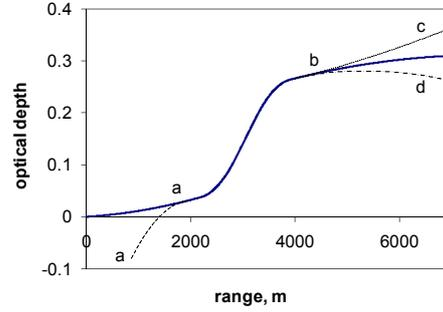
Fig. 4 – True optical depth (the thick solid curve) and possible near-end (curve *aa*) and far-end (curves *bc* and *bd*) distortions caused by the systematic lidar-signal distortions.
