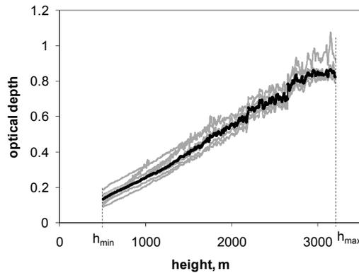
Fig. 5 – Profiles of  $\tau(0, h)$  (the thick black curve) and  $\tau_j(0, h)$  (the thin gray curves) measured during the Tripod Fire in Washington state.
