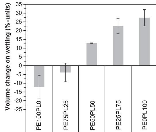
**Fig. 3 – Change of bale-dry sample volumes during wetting in cylinders from below ( $n = 3$ ) (mean  $\pm$  Sd).**
