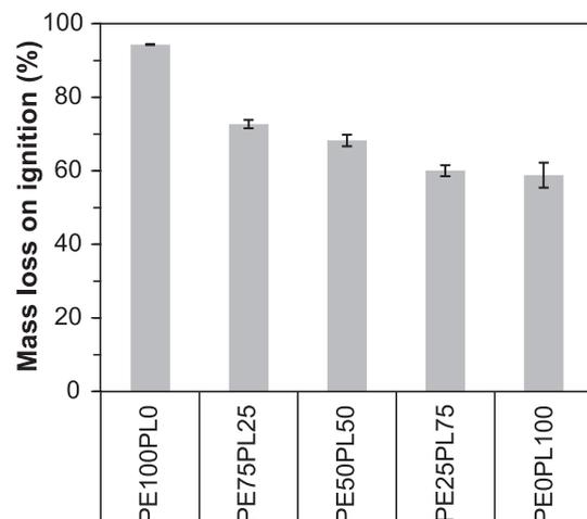
**Fig. 1 – Loss on ignition of the growing media (n = 5) (mean ± Sd).**
