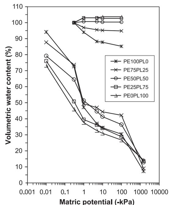
**Fig. 4 – Mean desorption water retention characteristics of the growing media in relation to the initial wet volume (means of  $n = 5$ ). The upper portion of the figure shows sample volumes in relation to the initial wet volumes ( $= 100\%$ ). An estimate of total porosity is plotted as water content at  $-0.01$  kPa, with air-filled porosity determined as total porosity less VWC at each matric potential.**
