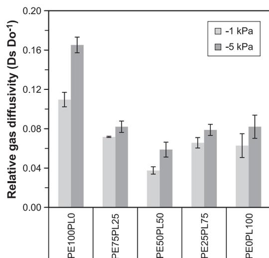
Fig. 5 – Mean relative oxygen gas diffusivity at  $-1$  and  $-5$  matric potentials according to Gislerod [29] ( $n = 3-5$ ) (mean  $\pm$  Sd).
