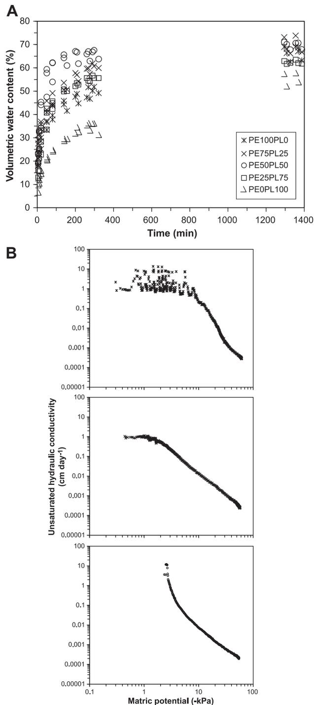
**Fig. 2 – Wetting of the growing media in cylinders from below ( $n = 3$ ); water content is expressed in relation to the initial bale-dry volume at the start (A). Unsaturated hydraulic conductivity ( $n = 2$ ) (B); top, middle, and bottom panels for PE100, PE75PL25, and PE50PL50, respectively.**
