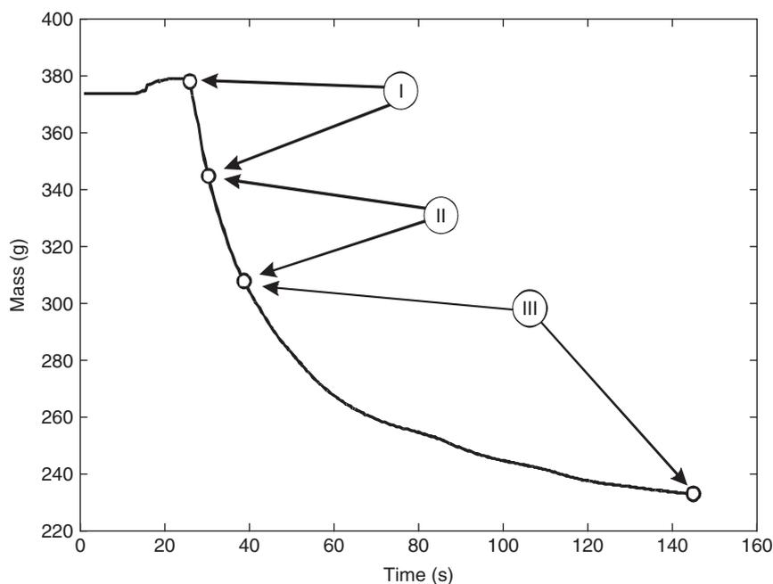
**Fig. 3.** Three main periods of burning can be identified in the mass loss data. Phase I is where ethyl alcohol is burned off. Phase II represents consistent external burning of the excelsior at a constant rate following complete combustion of the ethyl alcohol (constant slope). Phase III represents significant excelsior consumption where the excelsior fuel volume is decreasing and the interface between the excelsior and flame is no longer a vertical line.
