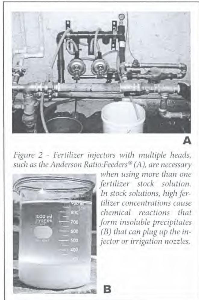
Figure 2 - Fertilizer injectors with multiple heads, such as the Anderson Ratio:Feeders® (A), are necessary when using more than one fertilizer stock solution. In stock solutions, high fertilizer concentrations cause chemical reactions that form insoluble precipitates (B) that can plug up the injector or irrigation nozzles.
