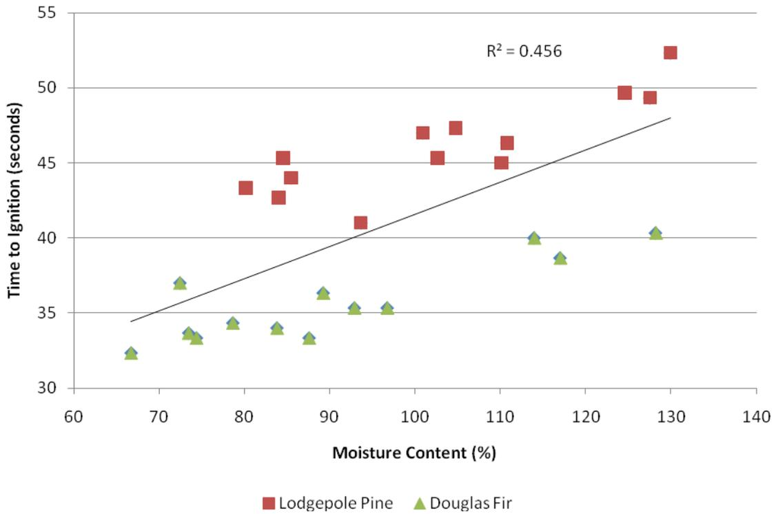
Figure 3 -- Time to ignition versus moisture content for Lodgepole pine and Douglas fir.
