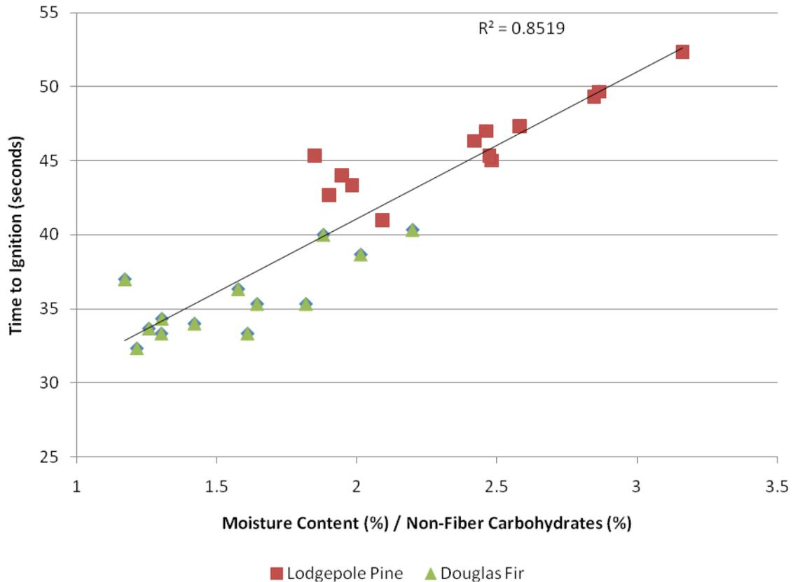
**Figure 5 – The ratio of moisture content and non-fiber carbohydrate percentage compared to time to ignition.**
