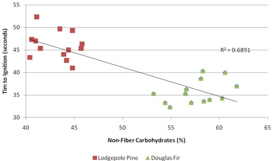
Figure 4 -- Time to ignition versus non-fiber carbohydrates for Lodgepole pine and Douglas fir.
