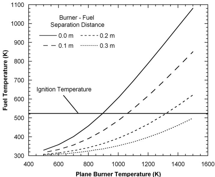
**Figure 8** Sensitivity of predicted fuel temperature to plane burner temperature. The ignition temperature indicated is the minimum temperature at which wood will ignite regardless of the heating arrangement (Babrauskas, 2003).
