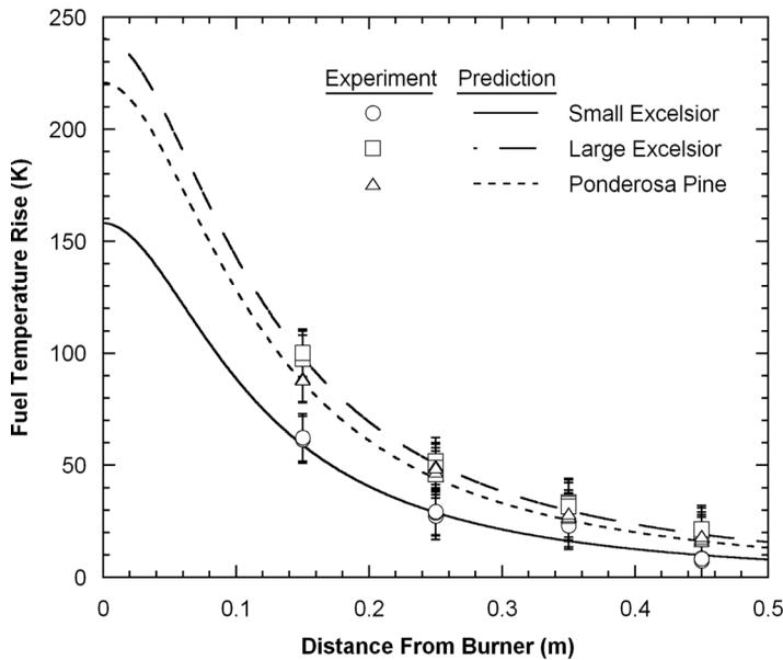
Figure 5 Comparison between model predictions and experimental measurements of fuel temperature rise.
