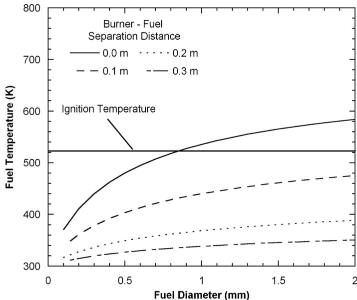
**Figure 9** Dependence of predicted fuel temperature on fuel diameter. The ignition temperature indicated is the minimum temperature at which wood may ignite regardless of the heating arrangement (Babrauskas, 2003).
