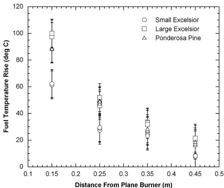
**Figure 4** Experimentally measured fuel temperature rise above ambient as a function of distance from plane burner for Ponderosa pine and small and large excelsior.
