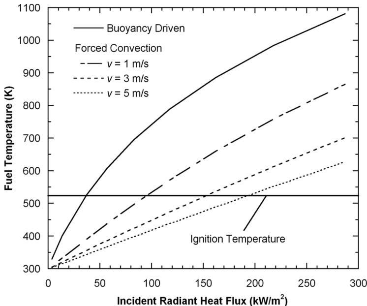
**Figure 7** Predicted fuel temperature as a function of incident radiation flux for different convective conditions. The ignition temperature indicated is the minimum temperature at which wood will ignite regardless of the heating arrangement (Babrauskas, 2003).
