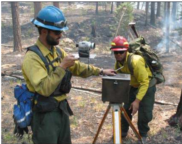
Figure 3--Fire researchers installing video acquisition box.
