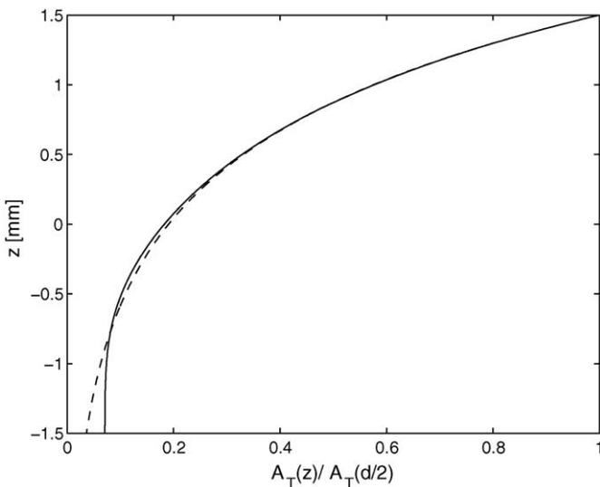
**Fig. 3.** Attenuation with depth of the normalized amplitude  $A_T(z)/A_T(d/2)$  of the temperature deviation from background temperature  $T_0$ , during one cycle of forcing ( $f = 0.05$  Hz,  $A = 10 \text{ W m}^{-2}$ ). The dashed line gives the theoretical attenuation curve, viz.  $\exp[-(d/2 - z)/\lambda]$ , where for this case  $\lambda = 0.905$  mm.
