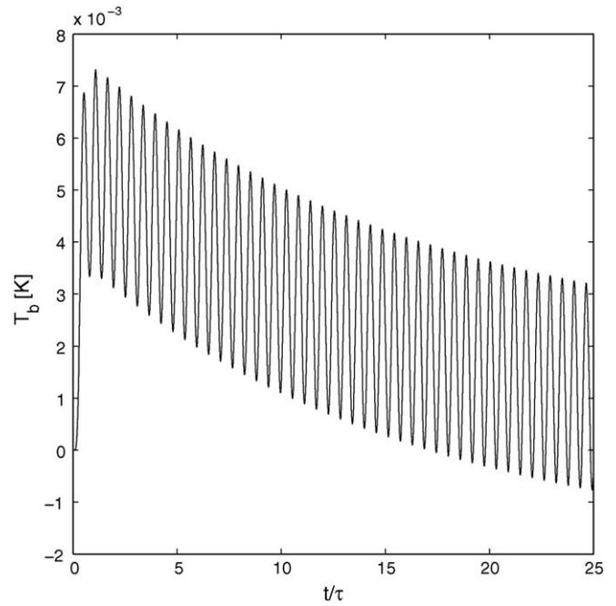
**Fig. 4.** Time variation of the temperature  $T_b$  at the base of the radiometer, with forcing frequency  $f = 0.05$  Hz and amplitude  $A = 10 \text{ W m}^{-2}$ . (The amplitude of the oscillation may be perceived as growing with  $t/\tau$ , however this is an optical illusion.)
