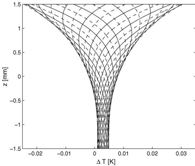
**Fig. 2.** Numerically simulated profiles of temperature deviation away from the background temperature  $T_0$ , during one cycle of forcing ( $f = 0.05$  Hz,  $A = 10 \text{ W m}^{-2}$ ) and plotted at intervals  $0.04/f$ . The amplitude of the temperature wave at the upper surface, determined from the ensemble of profiles at intervals  $\Delta t = 10^{-4}(1/f)$ , was  $A_u \equiv A_T(d/2) = 0.0275$  K.
