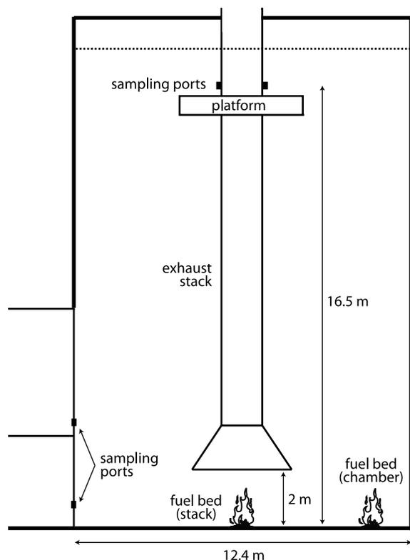
**Figure 1.** Schematic of the U.S. Forest Service Fire Sciences Laboratory combustion facility, located in Missoula, Montana. Image is to scale. The locations of the fuel bed and of the sampling ports during stack and chamber burns are indicated.
