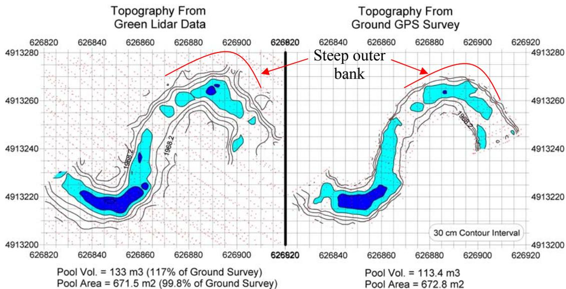
**Figure 3.** Comparison of topography mapped in the same pool-riffle channel reach with EAARL data (left panel) and survey-grade GPS (right panel). Red dots are points where elevation data were collected by each method. Notice the continuous EAARL data acquisition inside the channel and in the surrounding floodplain.
