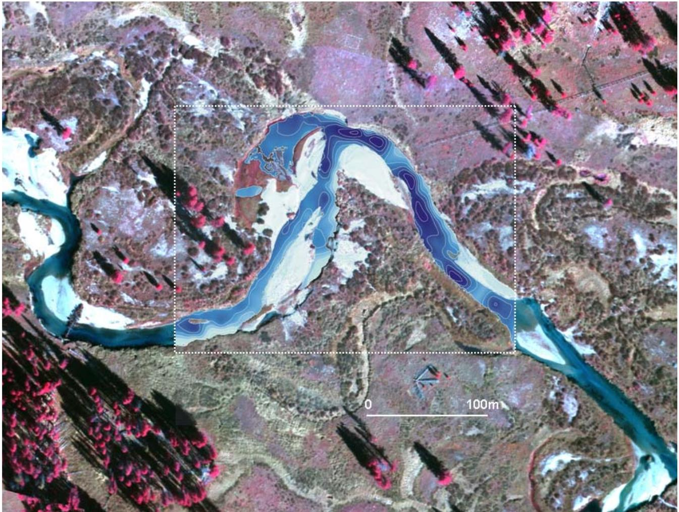
**Figure 8.** EAARL bathymetry of a portion of Elk Creek (bathymetry confined to area of channel within white box) overlaid on a mosaic of digital color-infrared imagery. The color-infrared imagery has not been rigorously ortho-rectified and co-registered to the bathymetry. The imagery and bathymetry were acquired simultaneously by the EAARL system. Bathymetric contours are at 50 cm intervals.
