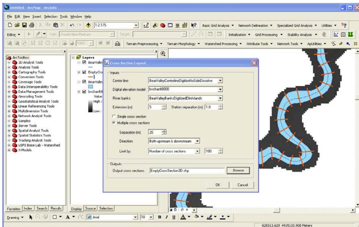
**Figure 9.** Screen capture of a web-based GIS tool being developed to automatically extract common channel and stream habitat metrics from EAARL data.
