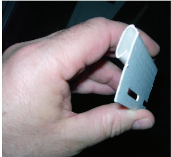
Figure 1. Side view of fence marker cut from vinyl undersill. Photo by Donald H. Wolfe
