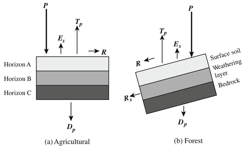
**Fig. 1.** Diagram showing the difference in primary hydrologic processes between typical (a) agricultural soil profile and (b) forest setting. The size of the arrows reflects the relative magnitude or rate of the individual processes:  $P$ , precipitation;  $T_p$ , plant transpiration;  $E_s$ , soil evaporation;  $R$ , surface runoff;  $R_s$ , subsurface lateral flow, and  $D_p$ , percolation through bottom of soil profile.
