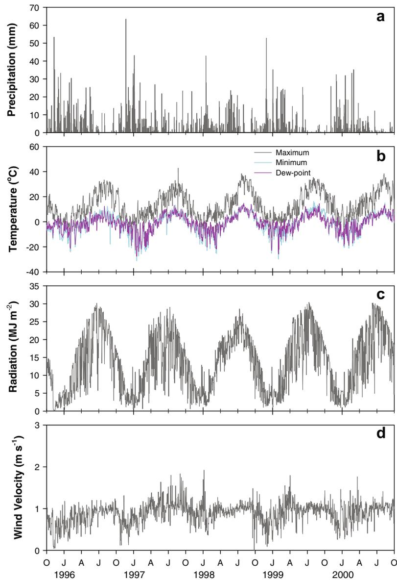
**Fig. 3.** Observed Hermada watershed daily weather inputs used in WEPP, (a) precipitation, (b) maximum, minimum temperature and dew-point temperature, (c) solar radiation, and (d) daily average wind speed.
