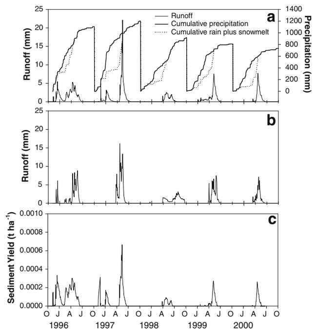
**Fig. 6.** Hydrograph and sedimentograph for the Hermada watershed. Daily watershed discharge (a) simulated by WEPP v2008.9 and (b) observed, and (c) daily sediment simulated by WEPP v2008.9.
