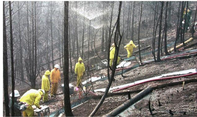
Figure 3. A photograph of the rainfall simulation experiment in progress. Three plots are visible in the photograph: the nearest plot is treated with a contour-felled log, the middle plot is untreated, the far plot is treated with a straw wattle
