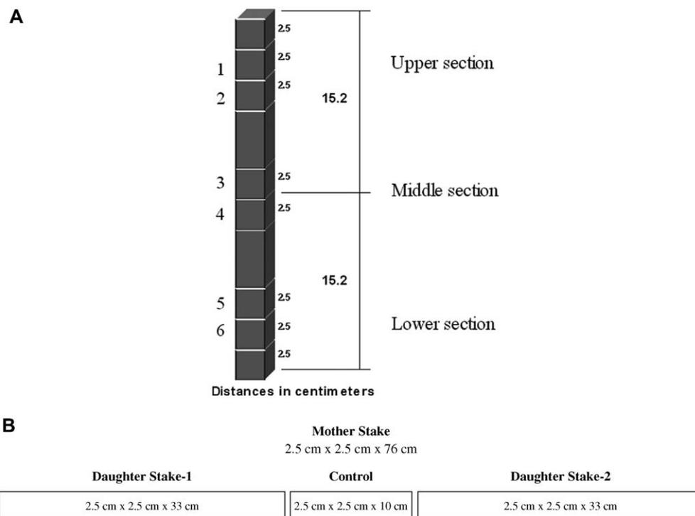
Fig. 1. Wood blocks used in laboratory wood strength tests (A) and wood stakes used in the European North–South temperature gradient study (B).
