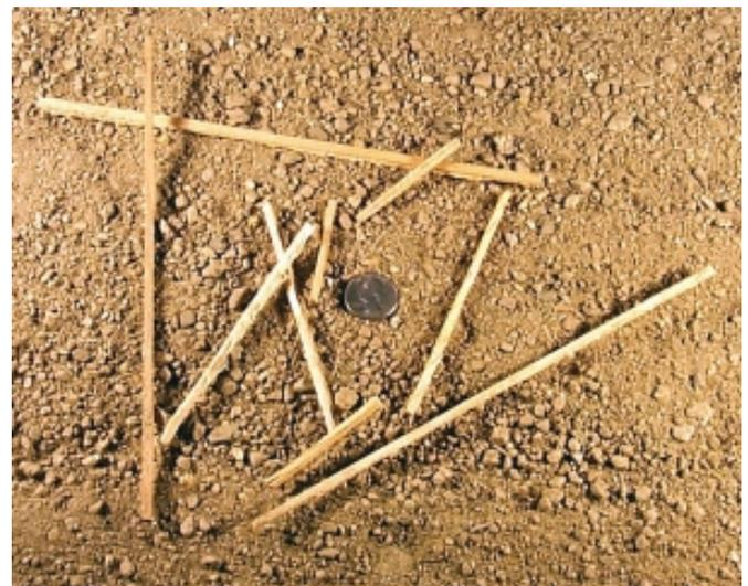
Figure 1—Narrow strips of wood veneer used as an alternative to straw mulch.
