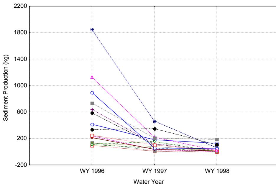
Figure 5. Erosion over the three-year study from each of the plots in Experiment 1 (length and slope) that operated all three years (N=14). All plots were treated at the beginning of WY 1996 by clearing the ditch and cutslope and grading the road surface. In WY 1996 differences are related to length times slope squared.
