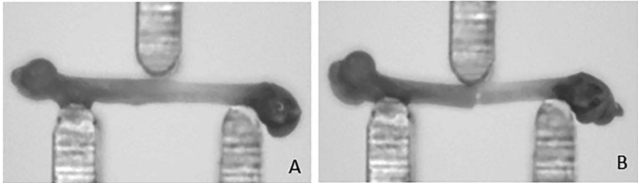
Fig. 1. Left femur of a little pocket mouse on a three-point bend fixture (A) prior to loading and (B) after fracture.
