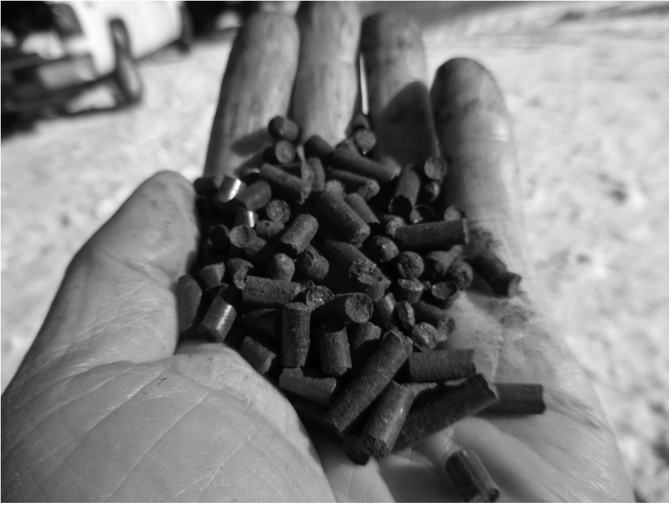
Figure 15.1. Pellets made from biochar and logging slash (photo by Deborah S. Page-Dumroese).
