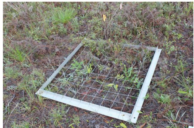
FIG. 3. The 10-cm  $\times$  10-cm grid coordinate system within a 1-m  $\times$  1-m aluminum frame used to create the coordinate grid to map the plants and fuels within our 1-m  $\times$  3-m plots. These are held in place with permanent steel rods driven into the soil at the corners of the frame. As the plants and fuels are mapped, the frame is moved up to the adjacent 1-m  $\times$  1-m treatment.
