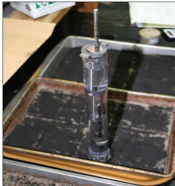
Figure 1. Tension infiltrometer on surface-applied biochar (5 Mg ha<sup>-1</sup> application rate) on granitic Inceptisol. Background pan is 10 Mg ha<sup>-1</sup> application rate.
