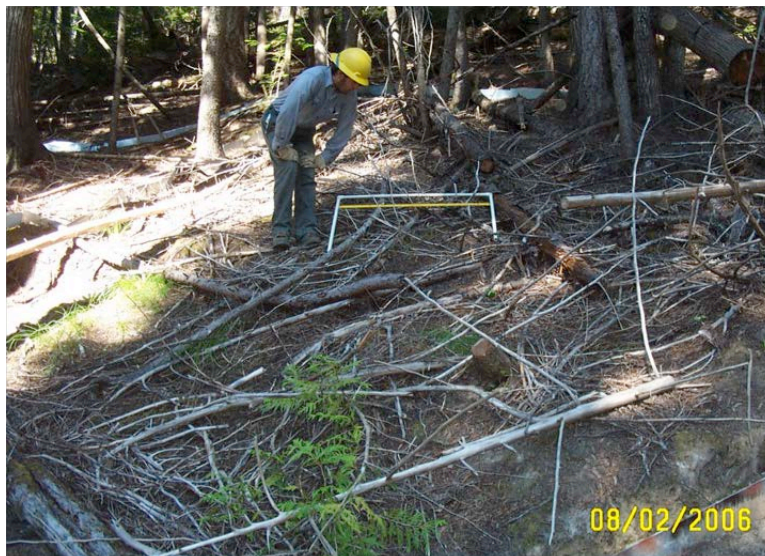
Forestry operations, such as thinning, can be a source of erosion, but to a lesser extent than roads and fire. RMRS scientists measure cover on a skid trail that has been covered with slash to minimize erosion risks. Photo by W. Elliot.
