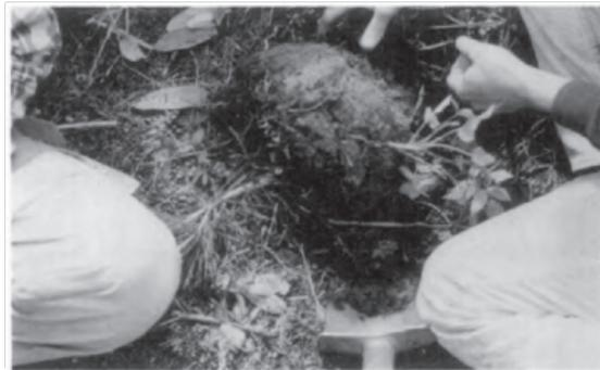
the soil by percussion. This method is fairly easy and can be used to characterize thin horizons. Replicate sampling is possible. However, driving in the cylinder can compress the
