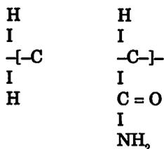
Non-cross-linked PAM, (hereafter designated as NC-PAM), trade named "Complete Green" (CG), is an anionic (relatively lower charged) polyacrylamide with a molecular weight of  $10\text{--}15 \times 10^6 \text{g/mol}$  (Aly and Letey 1988). This polyacrylamide was obtained from Complete Green Company (Los Angeles, CA).
