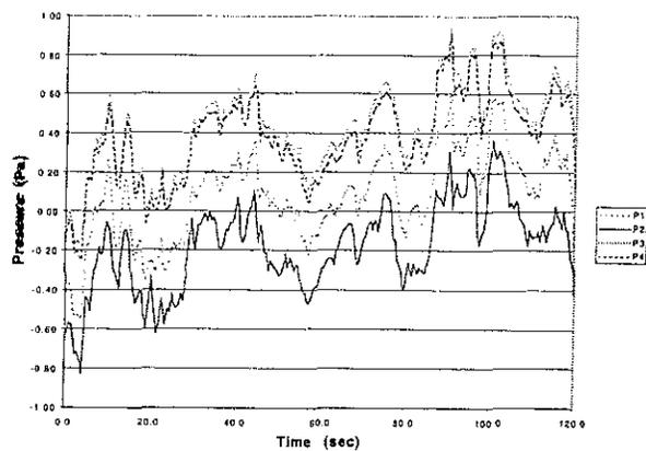
Figure 1. Time dependence of pressure fluctuations at the soil surface inside the LI-COR chamber (P1), at the surface outside the chamber (P2), at 10 cm soil depth under the chamber (P3), and at 15 cm soil depth under the chamber (P4).
