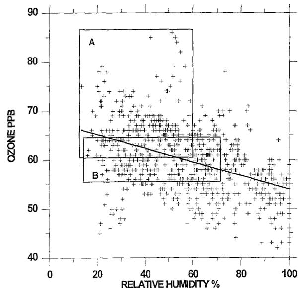
Fig. 6. Scatter diagram of hourly ozone concentrations vs relative humidity for the month of May, 1994 at the Brooklyn NDDN 10-m site. Box A includes ozone data during stratospheric-tropospheric intrusions; box B includes high daytime data not due to intrusions
