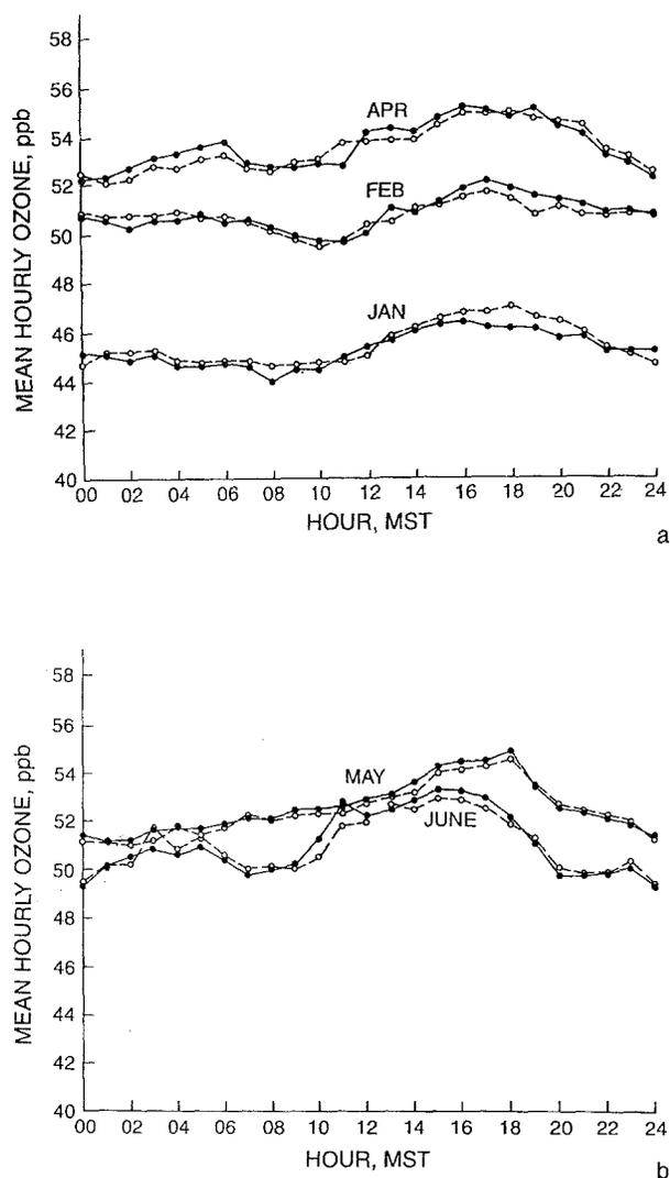
Fig. 3a, b. Comparison between mean diel ozone values for Brooklyn tower over the canopy (dashed lines) and Brooklyn NDDN (solid lines) for 1992. Figure 3a represents January, February, and April; Fig. 3b represents May and June
