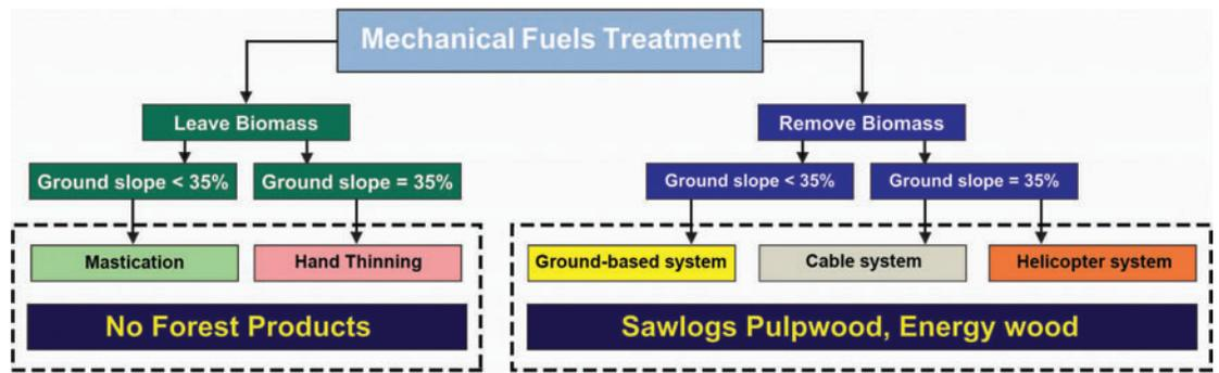
Figure 1—An overview of mechanical fuels treatment options as a function of slope.
