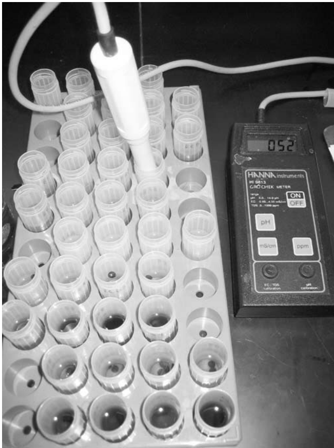
Figure 3 —For the freeze-induced electrolyte leakage (FIEL) trial, stem and foliar samples were placed in plastic vials containing 1.5 ml (0.05 oz) water and 0.25 g (0.9 oz) sand.
