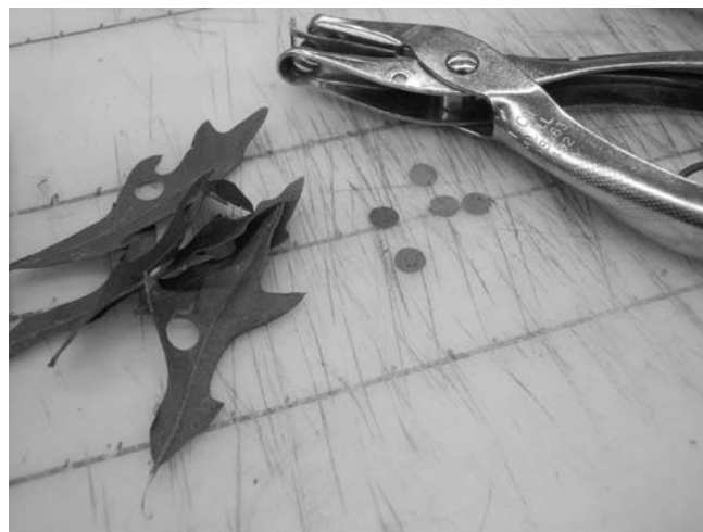
Figure 2 —Foliar samples for freeze-induced electrolyte leakage (FIEL) trial. One uniform disk was taken (midrib avoided) from each of five different leaves, taken from the middle portion of the shoot.
