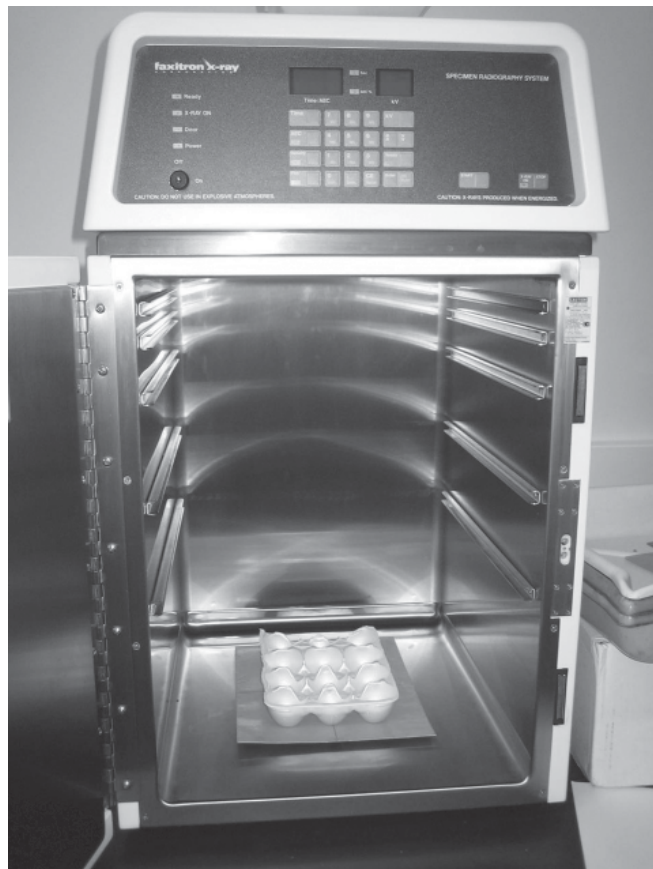
Figure 2 — Indented carton on top of photographic paper on bottom of X-ray machine.
