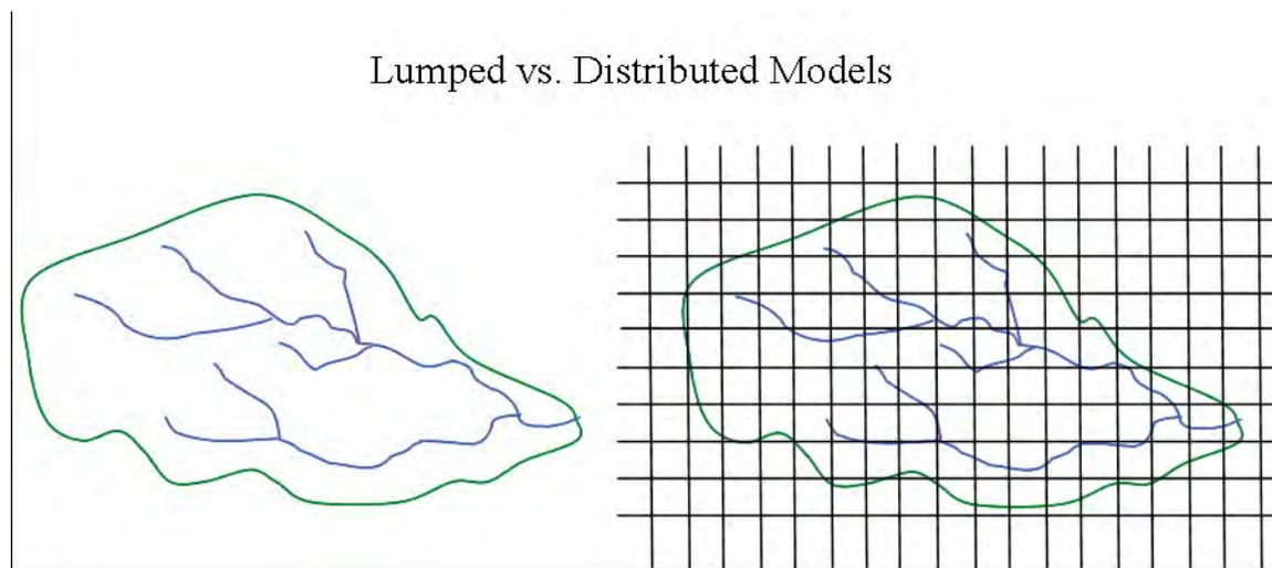
**Figure 1.** Lumped vs. distributed model. The “lumped” watershed on the left has a single value to describe soil, vegetation, and climate conditions in the entire watershed, whereas the “distributed” watershed on the right may have different values for each grid cell, or in some cases, individual hillslope polygons.
