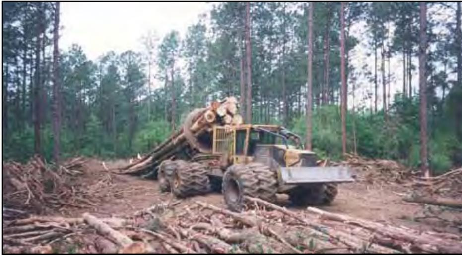
**Figure 6.** Clambunk skidder.
