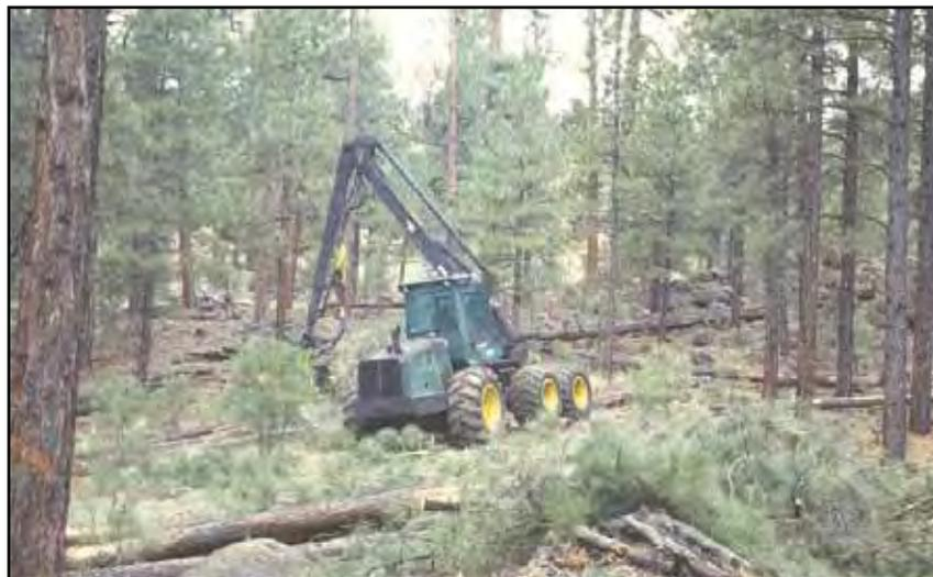
**Figure 5.** Wheeled harvester performing a fuel reduction thinning.
