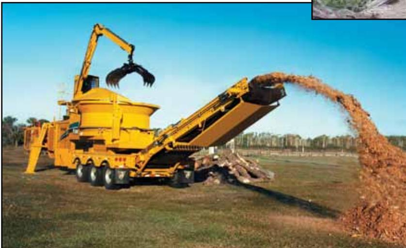
**Figure 9.** Tub grinder (Source: <http://www.collectiblereviews.net/>).
