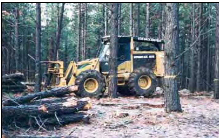
**Figure 3.** Wheeled feller-buncher thinning a ponderosa pine stand.
