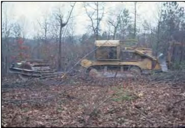
**Figure 1.** Drum chopper pulled by a bulldozer.
