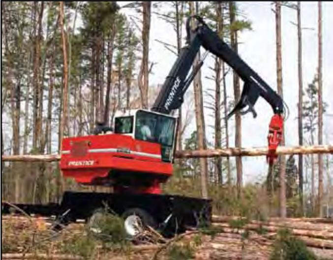
**Figure 7.** Knuckleboom loader (Source: <http://www.collectiblereviews.net/>).
