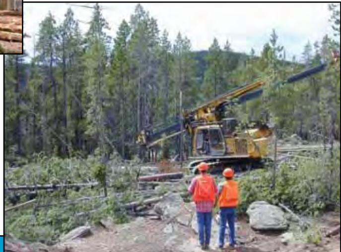
**Figure 8.** Strokeboom delimeter.
